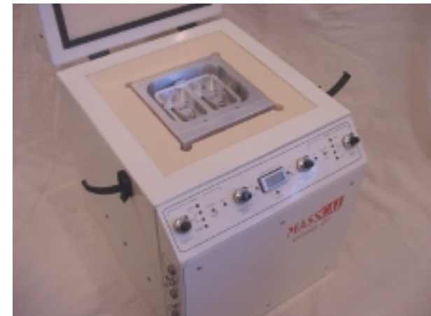
Figure 2 Top view of the Masscal G1 showing the sample chamber inside two layers of aluminum thermal shields, further insulated with several inches of high-quality polyurethane foam.
