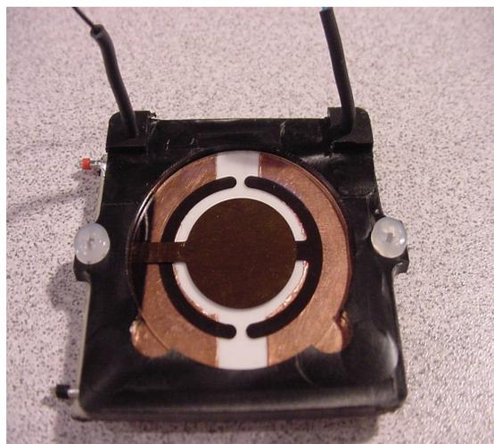
Fig. 2. A photo of the mass/heat flow sensor assembly in the Masscal QCM/HCC
