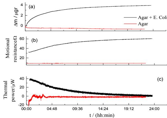
**Figure 8.** Changes in mass, motional resistance and thermal power when an agar film is inoculated and not inoculated with *E. coli* in air at 25°C, 50%RH.
