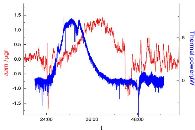
**Figure 11.** The rate of change of mass and thermal power when an agar film is inoculated with *E. coli*, anaerobically and then aerobically.
