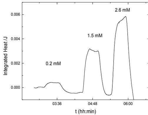
**Figure 6.** The integrated heat change for the adsorption/desorption of three concentrations of warfarin.
