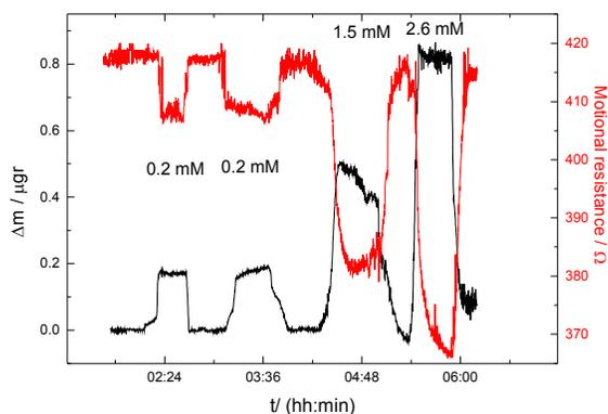
**Figure 2.** Changes in mass and motional resistance due to three concentrations of warfarin adsorption/desorption.
