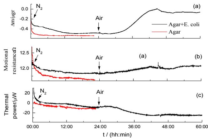
**Figure 10.** Changes in mass, motional resistance and thermal power when an agar film is inoculated and not inoculated with *E. coli*, anaerobically and then aerobically.
