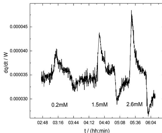
**Figure 3.** Changes in thermal power due to three concentrations of warfarin adsorption/desorption.
