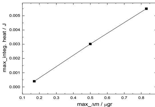
**Figure 7.** The dependence of the maximum integrated heat measured with the maximum “mass”change measured.
